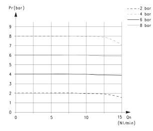
Pr = Outlet pressure (bar)\* Qn = Flow (NI/min)\*
