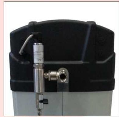
*The standard 10 minutes cycle is designed for full load operating conditions and the standard purge rate of 15% is normally "consumed" regardless of whether the dryer is operating on full or partial load. Considerable energy savings can be obtained by reducing this purge loss in proportion to the real working conditions.*
