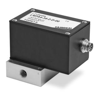
The servo valves LRPA4 are integrated servopneumatic systems for high precision pressure control loops in pneumatic systems. The devices include a 3/3-way servo valve size 4 resp. 6, a pressure sensor, an electronic PID-controller and the driver electronic for the servo valve. The valves are supplied with 24 VDC and an analogue command signal. There are an analogue output for the real output value and 2 binary outputs for additional system informations.
