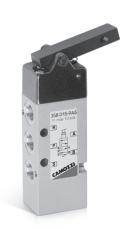
In order to facilitate the use of limit switch valves in applications where very low actuating forces and high flow rates are required, the Series 3 and Series 4 valves are equipped with new mechanical devices designed for this purpose. The Series 3 valve is designed with a mechanical lever which when operated releases an internal pilot signal to atmosphere. The sensitivity can be increased by adding a "whisker" or rod of Ø 3 mm to the lever.
