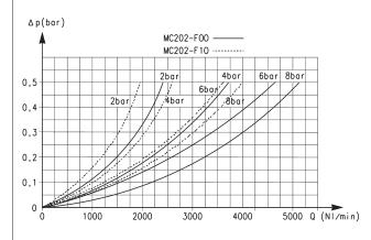
Flow diagram for models: MC202-F00 and MC202-F10
