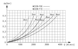
Flow diagram for models: MC238-F00 and MC238-F10
