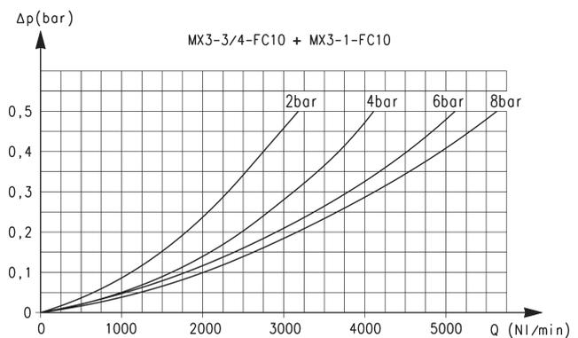
Reference diagram for models with filtering element = 0,01 µm
