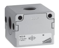
The take-off blocks, when equipped with a no return valve, allow the use of non lubricated air and should be inserted between the regulator and the lubricator. If mounted as last element, they should be assembled with terminal flanges.
