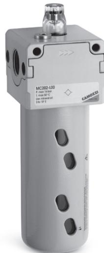
The Series MC lubricators are available with ports G1/4, G3/8 and G1/2. The bowls of these lubricators are made of metal and are equipped with a transparent viewer. The oil flow can be monitored through the small transparent cap and regulated by means of the proper adjusting screw.
